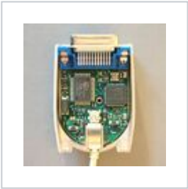
🔴 Agilent 82357A (Hardware-based, USB)
