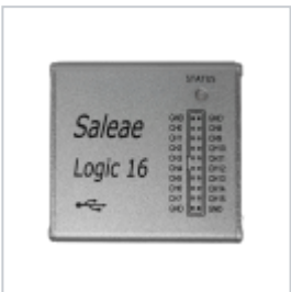
✓ mcupro Logic16 clone (16ch, 100MHz)
