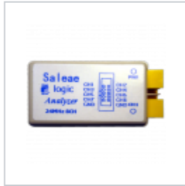
✓ MCU123 Saleae Logic clone (8ch, 24MHz)
