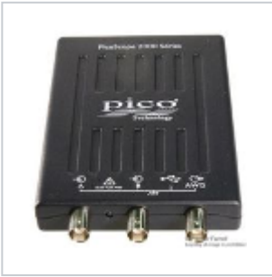
● Pico Technology PicoScope 2204A (100MS/s, 10MHz BW)
