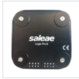
● Saleae Logic Pro 8 (4/8ch, 500/100MHz; 8ch analog, 50MSa/s, 5MHz BW)
