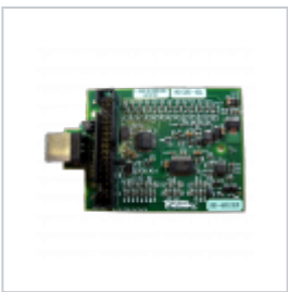
🔴 NI USB-6008 (8/2 analog inputs/outputs, 12 digital I/Os)
