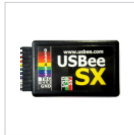
✓ CWAV USBee SX (8ch, 24MHz)
