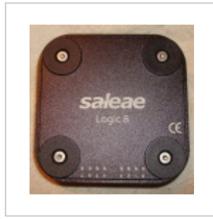
● Saleae Logic8 (3/6/7/8ch, 100/50/40/25MHz; 8ch analog, 10MSa/s, 1MHz BW)
