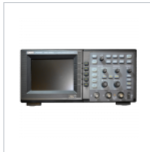
● UNI-T UTD2042C (2ch, 500MS/s, 40MHz BW)
