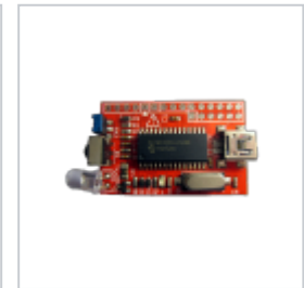
✓ Dangerous Prototypes USB IR Toy (1ch, 10kHz)
