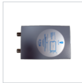
✓ SainSmart DDS120 (2ch, 50MS/s, 20MHz BW)
