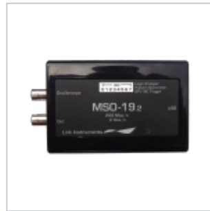
Link Instruments MSO-19 (8ch, 200MHz; 1ch analog, 200MSa/s, 60MHz BW)
