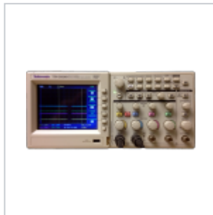
● Tektronix TDS2000B series (2-4ch, 1-2GS/s, 60-200MHz BW)
