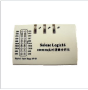
● Noname XL-LOGIC16-100M (16ch, 100/50/32/16MHz @ 3/6/9/16ch)
