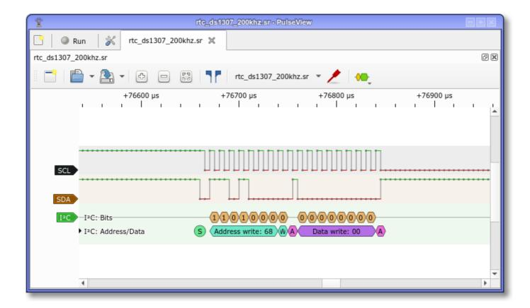
This is already very useful, and a massive improvement over counting out pulses on an oscilloscope screen. However, sigrok allows us to go one step further with the use of so-called stacked decoders.
