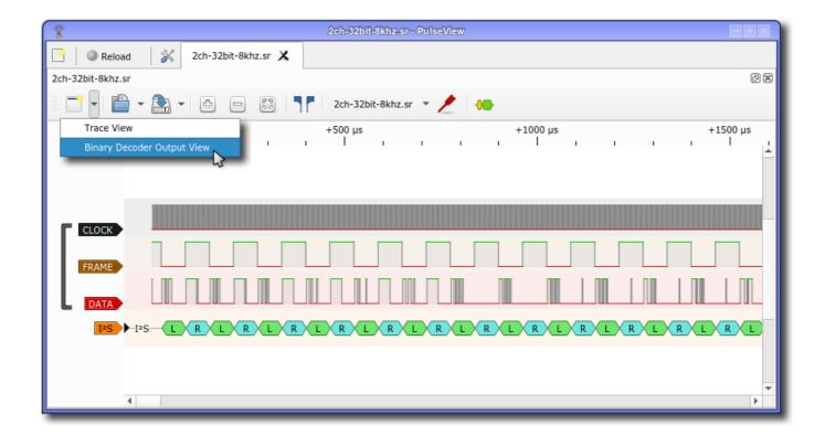
Once opened, you need to select a decoder with binary output for it to show anything - among which are I2C, I2S, EEPROM24xx, SPI and UART. Having acquired some I2S data and using the I2S protocol decoder lets you have the sound data as raw .wav file data, for example:
