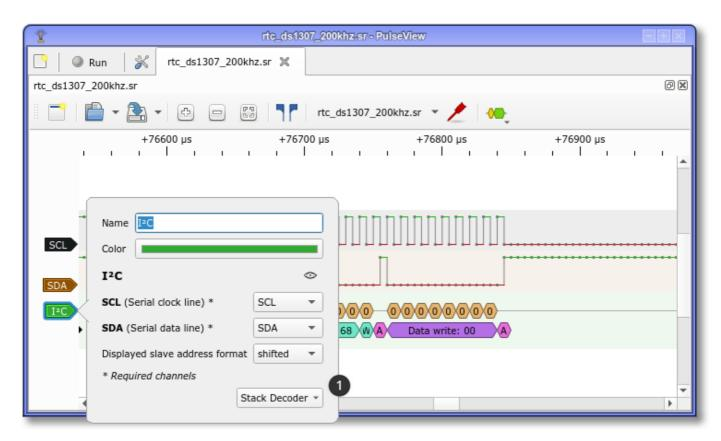
With the stacked decoder added, we can now see that PulseView has decoded the meaning of the I<sup>2</sup>C commands, so that we don't need to bother searching the reference manual. In this view, we can see that the I<sup>2</sup>C packet was a command to read the date and time, which was then reported to be "10.03.2013 23:35:30".
