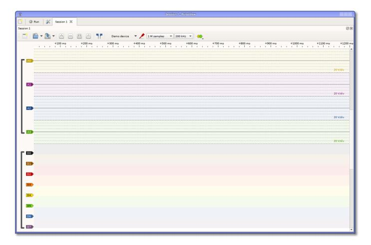
The PulseView user interface is geared towards navigation and analysis of captured waveforms, so the most space is by default used up by the main trace view. From here, you can access the most often used features.
