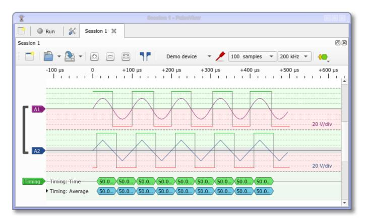
Here, A1 has been converted using a threshold (with default settings) and A2 has been converted using a Schmitt-Trigger emulation (also with default settings). Additionally, the conversion threshold display mode has been set to *Background* in the *Views* settings dialog. This way, you can tell how PulseView decided to change the logic signal level as you can now visually understand where the ranges for high and low are placed.
