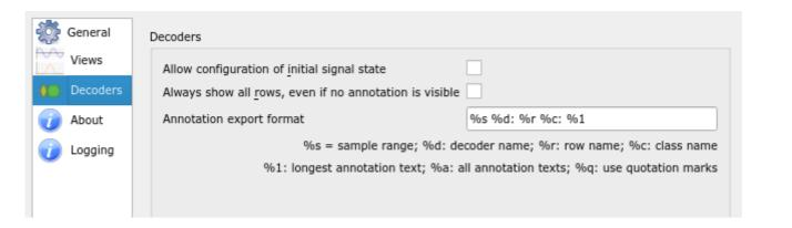
For example, the string "%s %d: %1" will generate this type of output for the DS1307 RTC clock protocol decoder: "253-471 DS1307: Read date/time: Sunday, 10.03.2013 23:35:30"
