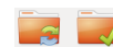
Figure 3.38: These symbols indicate the sync status of a file or folder. The Checkmark indicates that the file or folder has been synced, and the circular arrows indicate that the file or folder is in the process of syncing.
