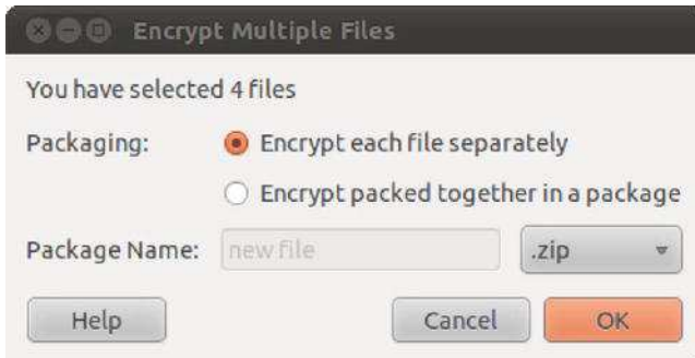
Figure 8-13. If you are encrypting multiple files, you can opt to encrypt each file or store all files in a compressed file and have that compressed file encrypted.
