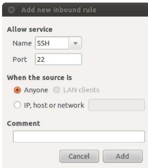
Figure 8-19. In the Add new inbound rule window, you can define new services to access your computer.
