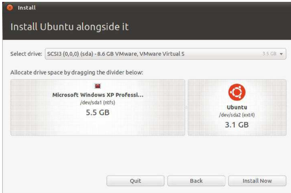
Figure 4-4. The installer will take as much space as Ubuntu needs, without shrinking the existing partition too much.
