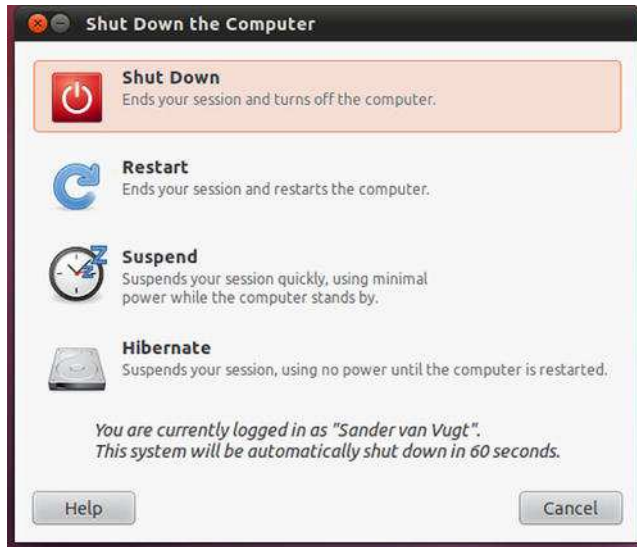
Figure 6-4. A variety of shutdown operations are available, some allowing for a quick resumption later on.
