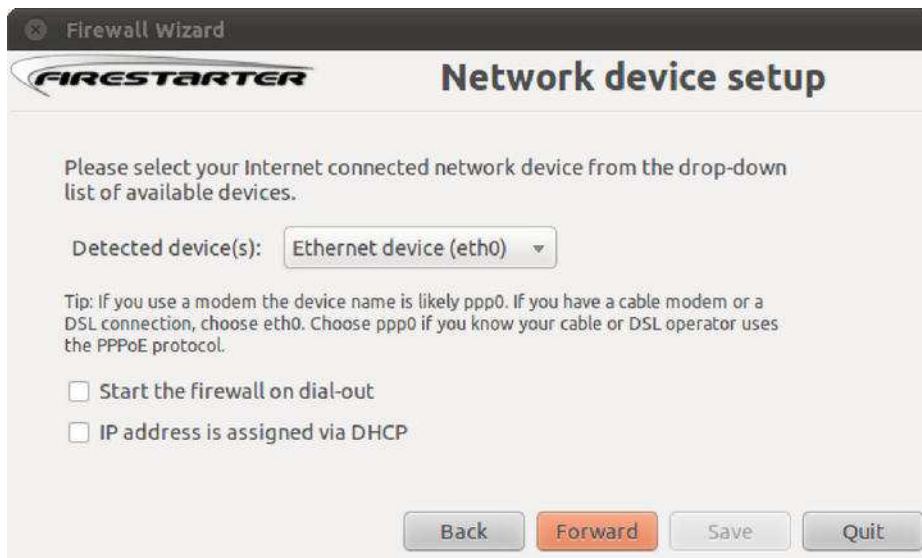
Figure 8-17. Firestarter includes a wizard to walk you through the basics of firewall configuration.
