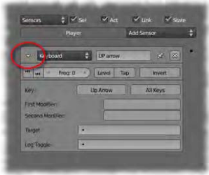
Figure 11–13. Completed “Up arrow” sensor with minimize button circled
