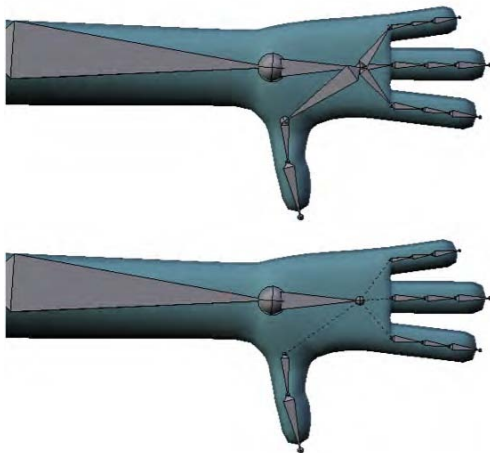
Figure 7–41. Delete the bones from hand to finger base. Dotted lines indicate that the finger bones are still parented to the hand bone.
