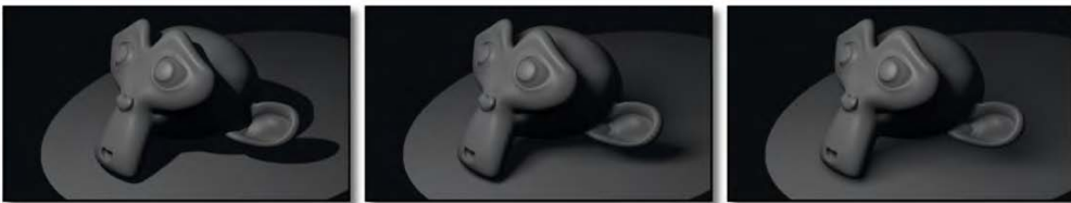
Figure 4-14. Different Soft Size values applied in the shadow settings of a spotlight
