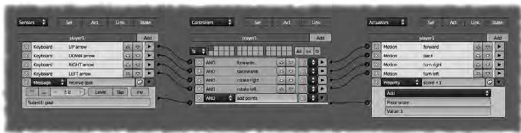
Figure 11–35. player1 is set up to add the score on receiving a message from the ball.
