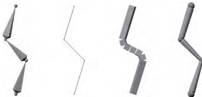
Figure 7-28. Different display types for bones (from left to right, octahedron, stick, B-bone, and envelope)
